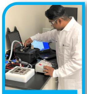
The Guarded Hot Plate determines heat flux, indicating the comfort characteristics of your foam using Alexicool<sup>®</sup> FM.
